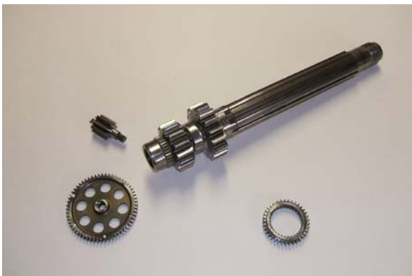
Figure 4. Oil pump drive components
